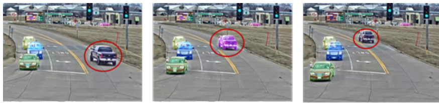
Figure 8: ID Switch Happens as Tracking by Masks. Obviously, this Is because the Lack of Stability of the Segmentation Algorithm. To Further Fix this, A Combination of Bounding Box and Segmented Mask should Be Proposed.
